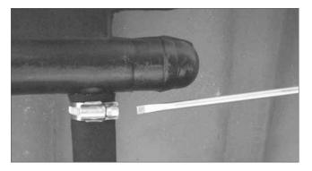
To use the end stopper set for closing off connections with a diameter of 25 mm that are not needed, first fasten the fabric hose with hose clamps.
