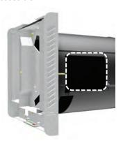
5. Remove the PVC cover of the control board at the side of the ribbon cable entry out of the slot on the EPP housing, and gripping the plug, cautiously pull the ribbon cable out of the UI X9 plug connection on the control board.
