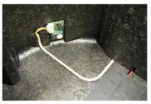
8. Connect the sensor cable to the clamping point SENSOR X8 on the control board.
