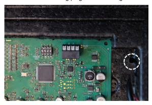
7. Guide the sensor cable, together with the wire ends, from the inside to the outside through the cable guide of the EPP housing, and push the sensor cable into the cable recess.
