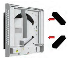
8. Put the interior top cover onto the bottom cover, and press them in the area of the locking connections until you can hear them engage.
