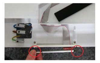
3. Disconnect the ribbon cable from the board for the control panel, by pulling the ribbon cable's plug (gripping with two fingers) out of the socket located on the board. Meanwhile, hold the control panel tight in the area of the plug connection using two fingers on your other hand. Remove the ribbon cable from the cable retainers and guide it back to the opening and into the bottom cover of the interior cover.
