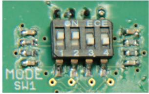
Fig. Position of DIP switch, factory setting
