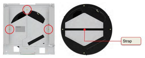
7. Gripping the strap, cautiously pull the enthalpy exchanger out of the EPP housing.
