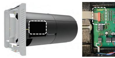
3. Undo the four nuts used to fasten the bottom cover of the interior cover to the EPP housing from the threaded bolts, and remove the bottom cover including the electronic equipment cover.
