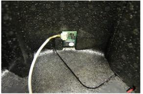
6. Remove the blanking plug for the cable guide in the vicinity of the control board from the EPP housing.
