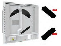
4. Gripping the pulling tabs, pull the filter carefully out of the filter compartment.
