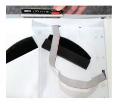
6. Install the ribbon cable in the designated fixing points, taking care to produce a smooth overlapping in the vicinity of the 90° bends. Then snap the control panel onto the control panel carrier in the correct position.
