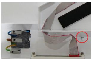
Cautiously pull the control panel using the two interlocking fixings (at the side) off the control panel carrier, and guide the control panel, together with the still connected ribbon cable, out of the control panel carrier for better handling.
