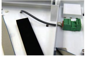
4. Connect the wires of the connecting cable to the BUS X7 terminal on the control board.
