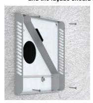
Press the top cover for the outside wall panel onto the bottom cover using all four locking connections. Fasten the four screws from the supplied installation kit for the top cover of the outside wall panel on the bottom cover of the outside wall panel.
