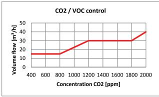
Diagram 2: Factory setting characteristic curve for Automatic operating mode with CO<sub>2</sub> / VOC control
