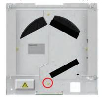
If necessary, a suitable tool can be used to remove the centring spring raised 5 mm, and arranged 3 times on the EPP housing, to the dimension Ø 300 of the EPP basic body, in order to facilitate the insertion!
