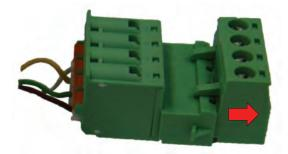
Connect the four wires of the on-site cable (J-Y(ST)Y 2x2x0.6) for the external control panel to the plug-in connector part with the screw-type terminals.
