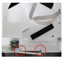
5. Guide the ribbon cable through the frame opening of the bottom cover and the control panel carrier. Restore the plug connection between the ribbon cable and control panel.
