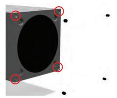
2. Using the raised contours for the airflow, put the bottom cover of the outside wall panel onto the EPP housing, and fasten it on the four fixing points on the wall mounting pipe.
