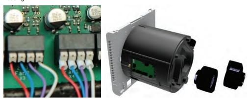
6. The structurally identical fans can be removed from the EPP housing after the fan cables have been disconnected from the FAN1 X4 and FAN2 X3 terminals on the control board, whilst feeding in simultaneously. In doing so, do not damage the sealing tapes in the vicinity of the fans.
